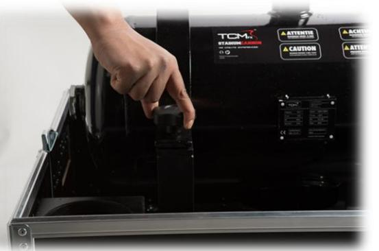
Connect a compressor with a hose to the tank of the Stadium Cannon, Warning! The Maximum output pressure is 8 bars. (Compressor is not included)
