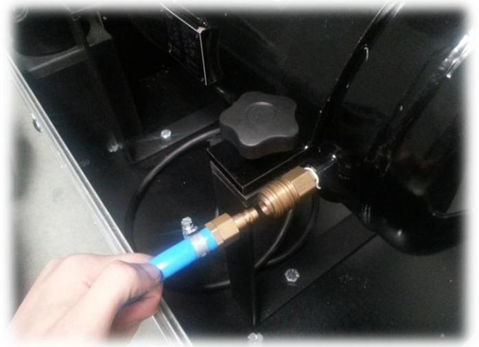
Connect a compressor with a hose to the tank of the Stadium Cannon. Fill the tank with pressure until the pressure gauge indicates it has reached 8 bars. You can now disengage the compressor if necessary. Remember to always check the pressure gauge! If it is above 8 bars, you can always vent through the vent valve.
